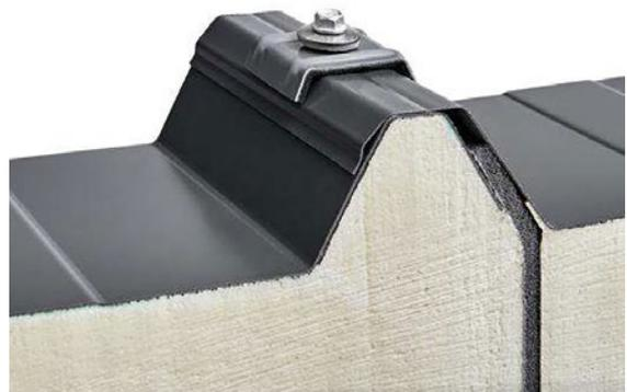
The offer of Balex Metal also includes the so-called stress redistributors that minimize the risk of damage to the linings in the locks by distributing the load from the pressure of the fasteners through this plate to the lining. This is an exceptionally advantageous solution when installing wall panels with invisible fastening.
