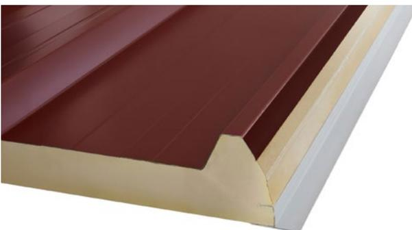
When mounting PIR FIBER sandwich panel it's necessary to remember about h-profile and filling the gap between the core and this profile with PUR foam (recommended).
